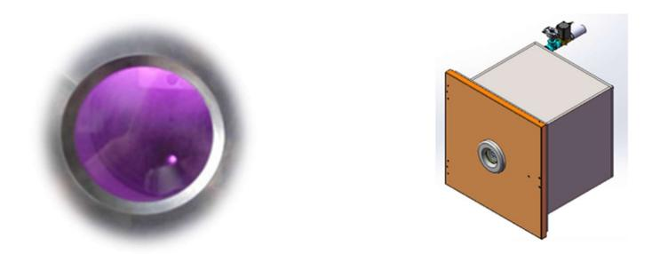
Figure 6: Vacuum Plasma Chamber, 0.064 Cubic Meters
