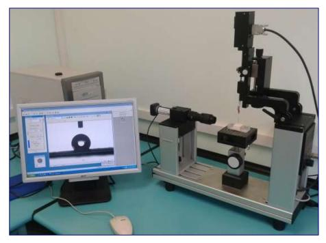
Figure 4: Optical Tensiometer
